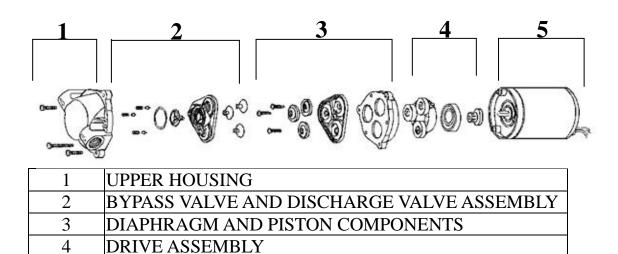
MOTOR ASSEMBLY (LESS BASE PLATE)
