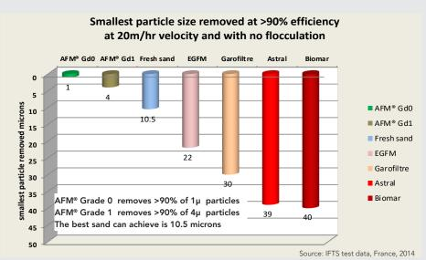
Sand was 16/30 Leighton Buzzard sand. AFM®grade 0 performance at 4 & 10 micron against water flow velocity 100 10 micron AFM Grade 1 Performance at 4 & 10 micron against water flow velocity AFM 10 micron 4 micron 90 Performance % AFM 4 micron 70 60 10 15 20 Water flow m/hr sand 4 microns 30 Water flow m/hr
