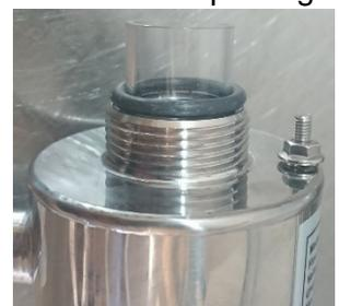
3. Place the o-ring over the exposed end of the glass thimble and seat the o-ring firmly against the thread **as shown beside.**
