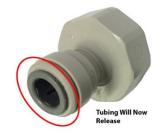
tubing from push-fit fittings, depress the floating collet (shown to the right), then pull the tubing out.
